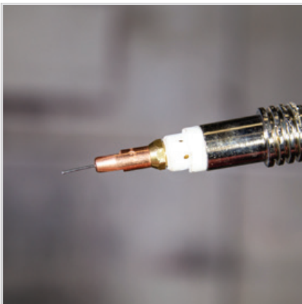
(12) Fit the correct size contact tip over the wire and fasten tightly into the tip holder.
