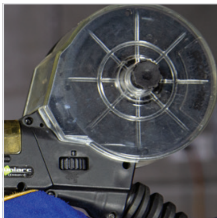
(7) Push the cover release button to unlock the wire feed /spool cover.
