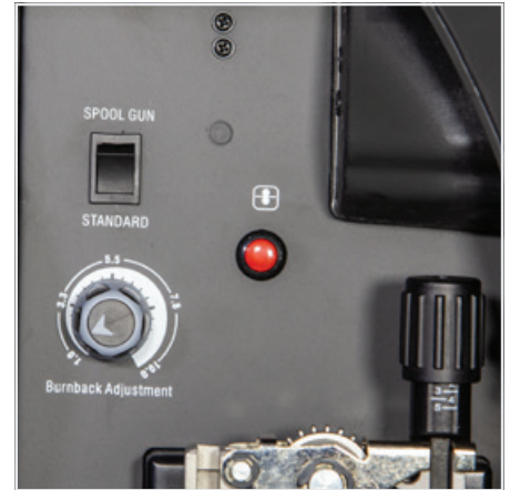
(11) Press and hold the inch wire button to feed the wire down the torch cable through to the torch head.
