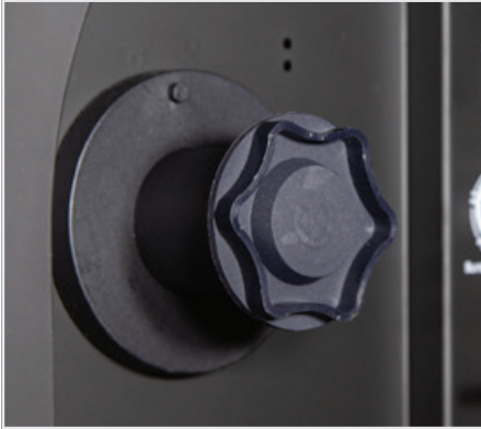
(1) Remove the spool retaining nut.
