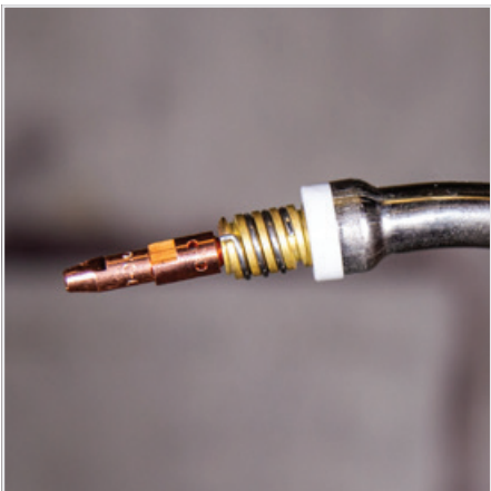
(16) Fit an Aluminium contact tip of the correct size to match the wire diameter being used
