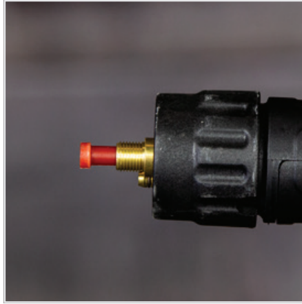
(2) Remove the liner retaining nut
