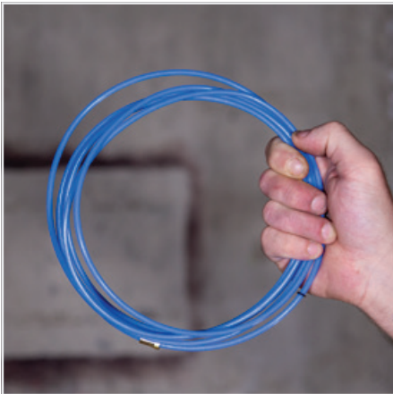
(4) Carefully unravel the new liner
