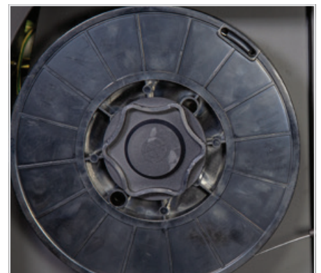
(9) The weight and speed of the wire spool turning creates an inertia that can cause the spool to run on and the wire loop over the side of the spool and tangle. If this happens increase the pressure on the tension spring inside the spool holder assembly using the tension adjustment screw.
