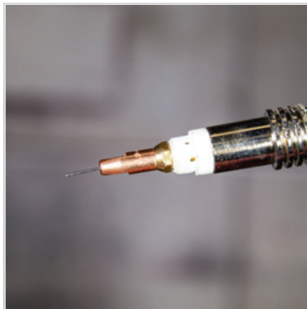
(13) Fit the correct size contact tip over the wire and fasten tightly into the tip holder.
