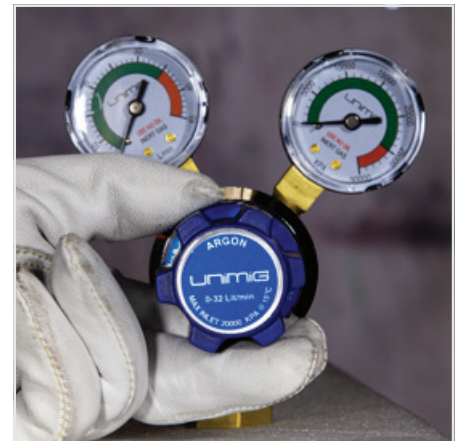
(14) Carefully open the valve of the gas cylinder, set the flow to 8-10 L/min
