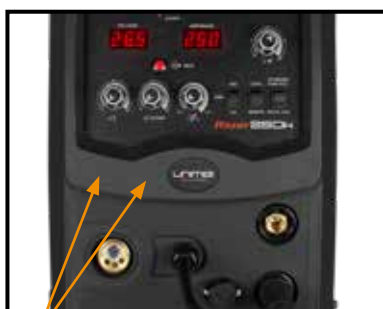
(15) Set welding parameters using the voltage and wire feed controls.
