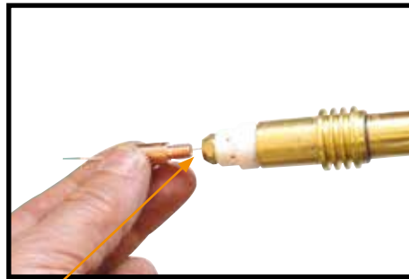
(13) Fit the contact tip over the wire and screw it into the tip holder, nip it up tight.
