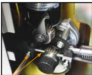
(10) Loosen the inlet guide tube retaining screw.
