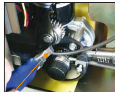
(15) Cut the extended Polymide liner with a sharp Stanley knife just in front of the drive roller
